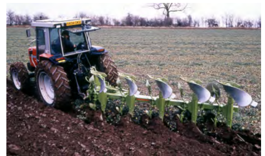
Good ploughing is dependent on correct set-up, effective use of skimmers and favourable soil conditions.
