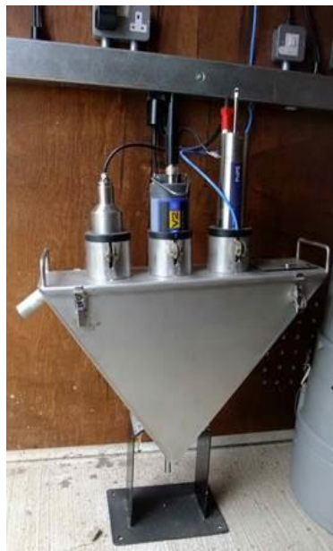
Figure 7. By-pass flow cell
