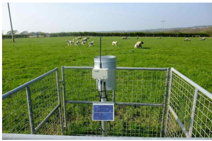
Figure 9. Soil moisture station with tipping bucket rain gauge
